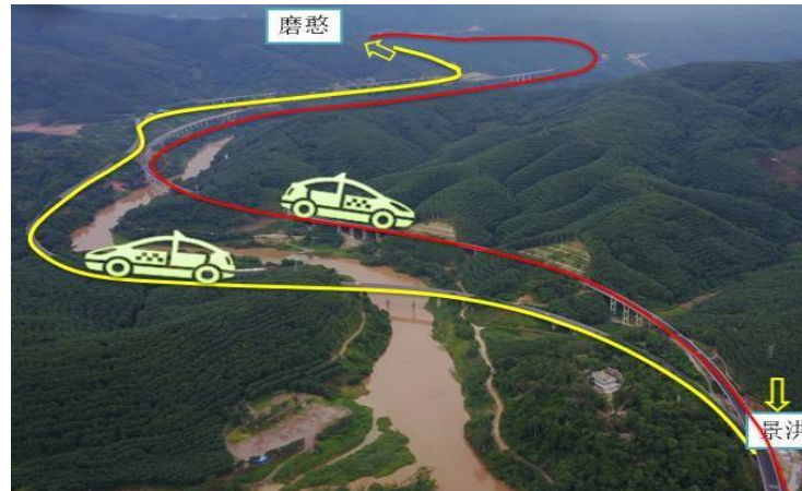
Fig. 4.1 Interweaving between upslope and downslope on new and original subgrade separated in large spacing (Red line: downslope on new subgrade; yellow line: upslope on original subgrade)
