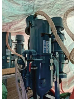
Fig. 37 Environmental friendly self-priming sand washer
