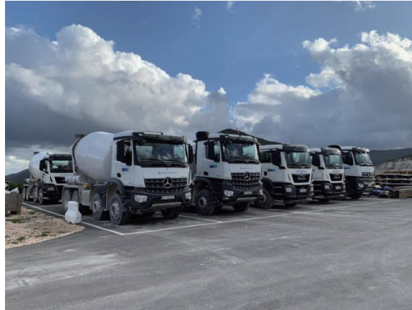
Fig. 39 Asphalt overlay for the parking area of concrete tank truck to prevent oil leakage from polluting the land
